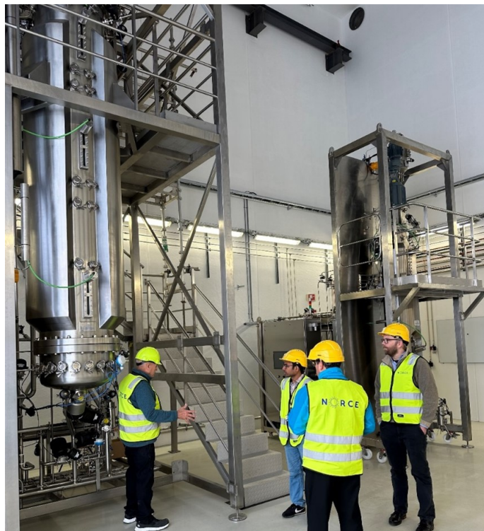
Pilot-scale gas bioreactors at project partner NORCE in Stavanger, Norway, October 2023
