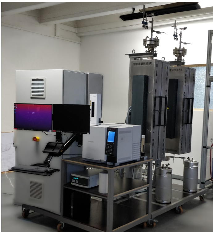
First-stage chemo-catalytic acetone conversion pilot unit at project partner RANIDO in Czech Republic
